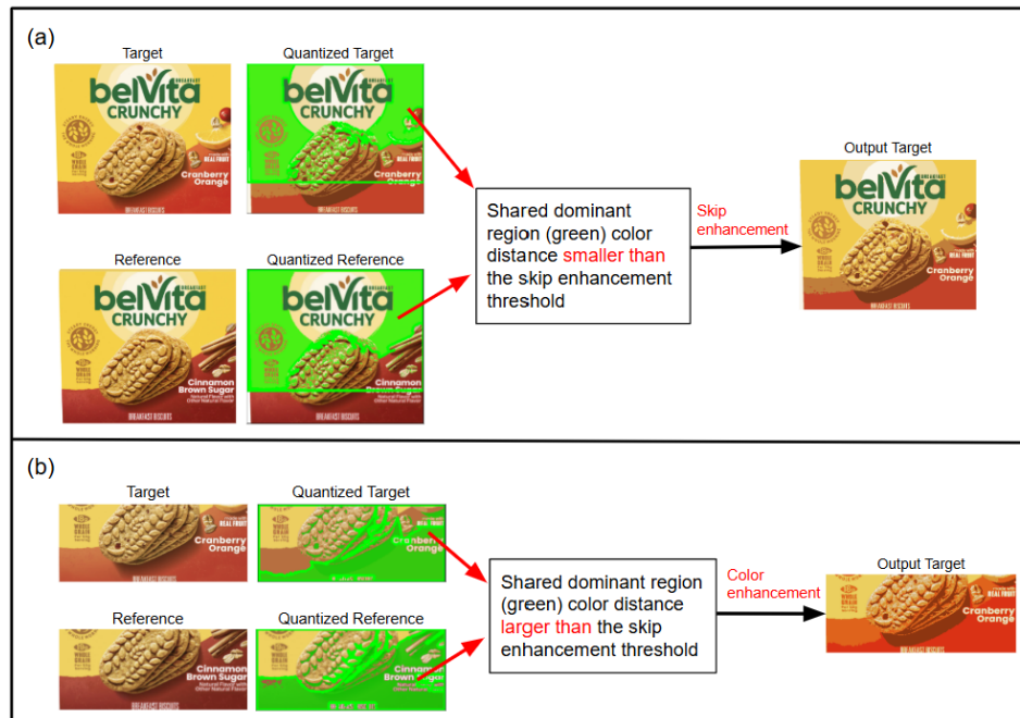
Figure 14: Effect of the color-enhancement algorithm on real-world objects with multiple color regions, illustrated using two BelVita cookie packages. (a) With full packages, the algorithm selects the shared yellow header as the dominant region. Since the color distance of the shared dominant region between target and reference is below the enhancement threshold, enhancement is skipped, and the target proxies remain visually similar to the reference. (b) With only the lower halves, the dominant regions (orange vs. red) differ more, exceeding the threshold and triggering enhancement, making the target proxy more distinguishable to the reference.
